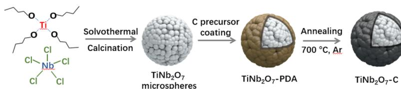
**Figure 2.** Synthesis schematic of the TNO-C materials.
